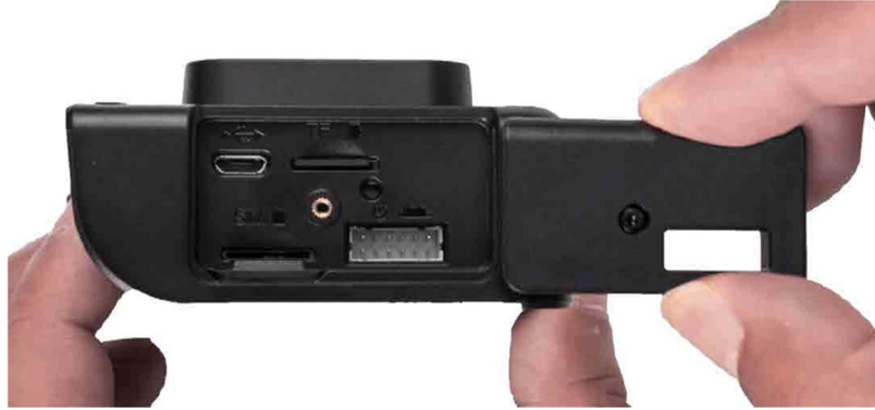
Removing the right panel I/O cover
