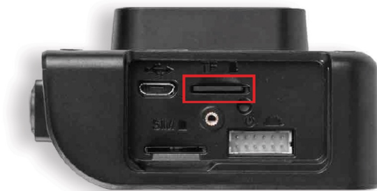
Locating the Micro SD card slot
