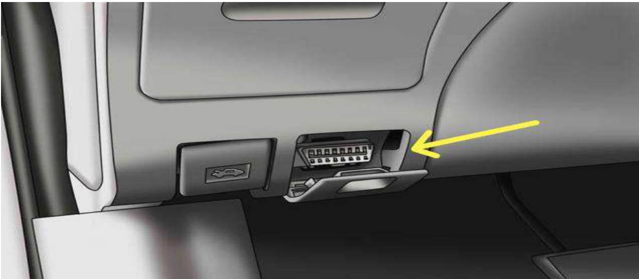
General Positions of OBD Port of Different Vehicle Models
