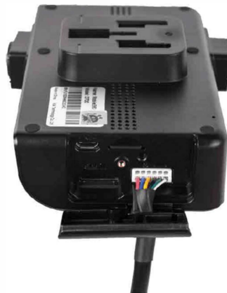
Plugging in the 12-pin connector of the OBD II Power Cable
