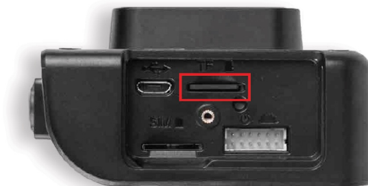
Locating the Micro SD card slot
