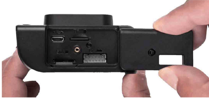
Removing the right panel I/O cover
