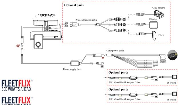
Schematic Diagram of System Connection-Power Supply through Standard Power Cable
