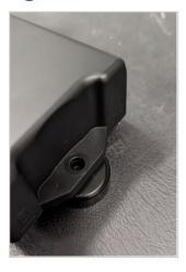
Using a #2 Phillips screwdriver, insert the 3/8" long, thread locking screw through the enclosure and into the magnet.
